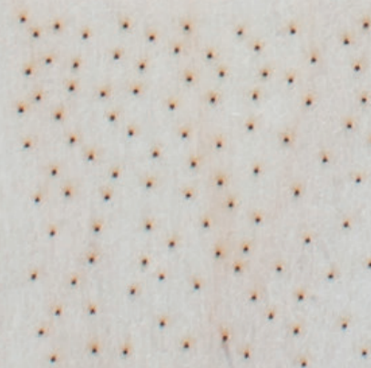
origine pattern (o.p.) : round, 0,433 mm, disposition, random, forming a square, 60 mm.
